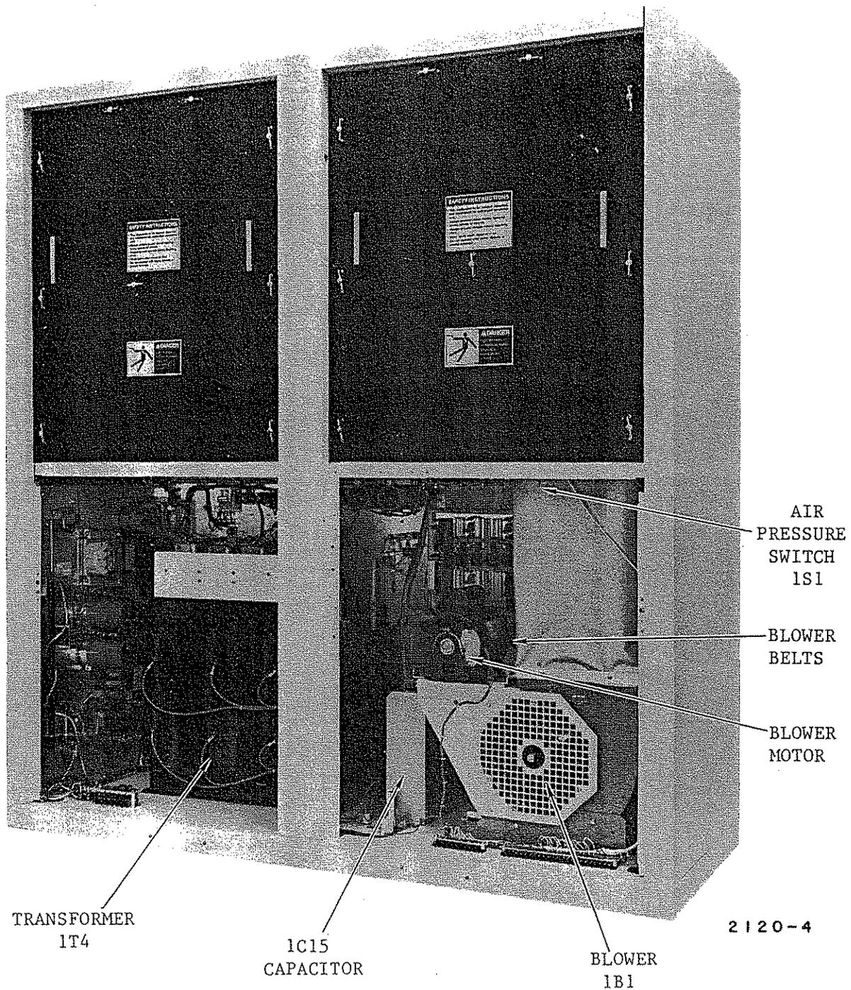
Figure 2-2. Transmitter Component Locations (Sheet 1 of 4)
