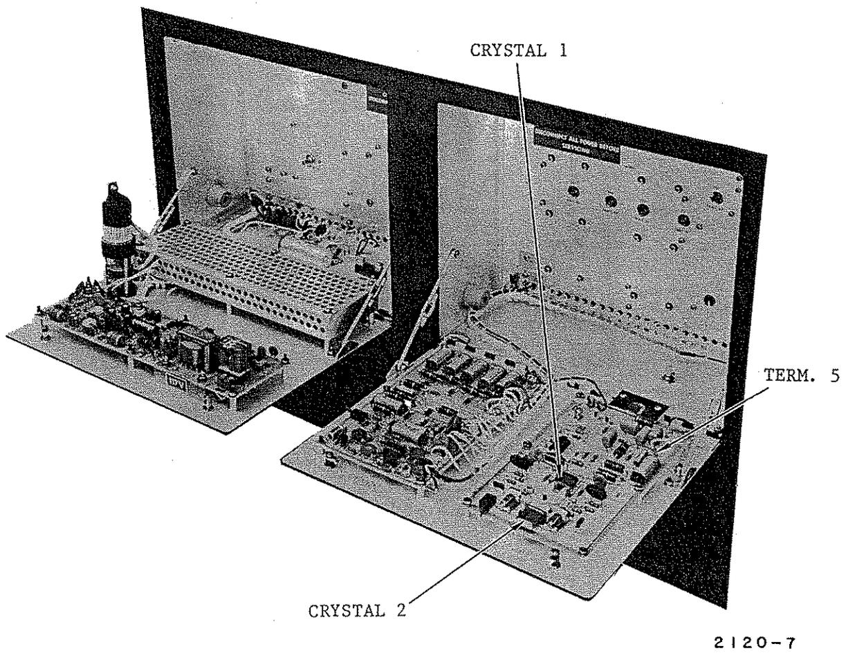
Figure 2-2. Transmitter Component Locations (Sheet 4 of 4)
