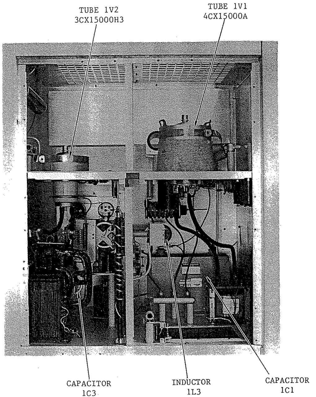
Figure 2-2. Transmitter Component Locations (Sheet 2 of 4)
