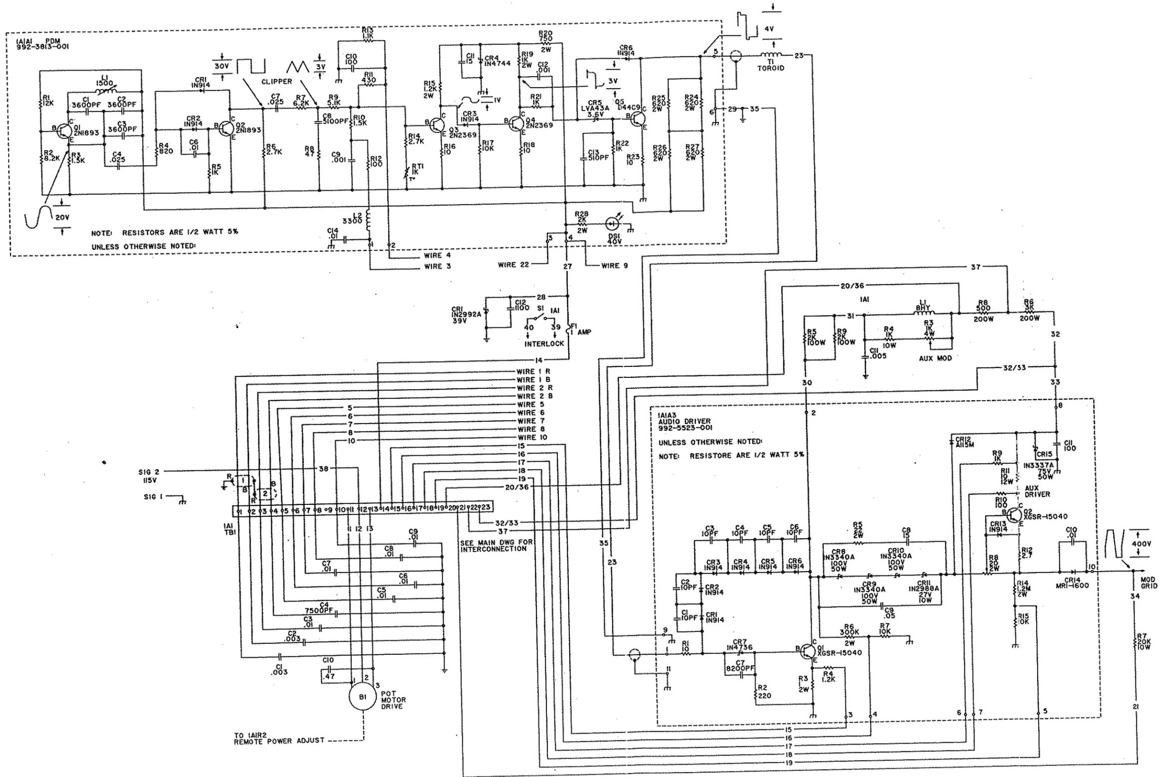
FIGURE 8-8. PDM CHASSIS SCHEMATIC
