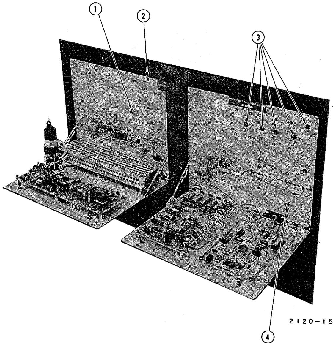
Figure 3-7. PDM Chassis 1A1 and RF Driver and Overload 1A2, Controls and Indicators
