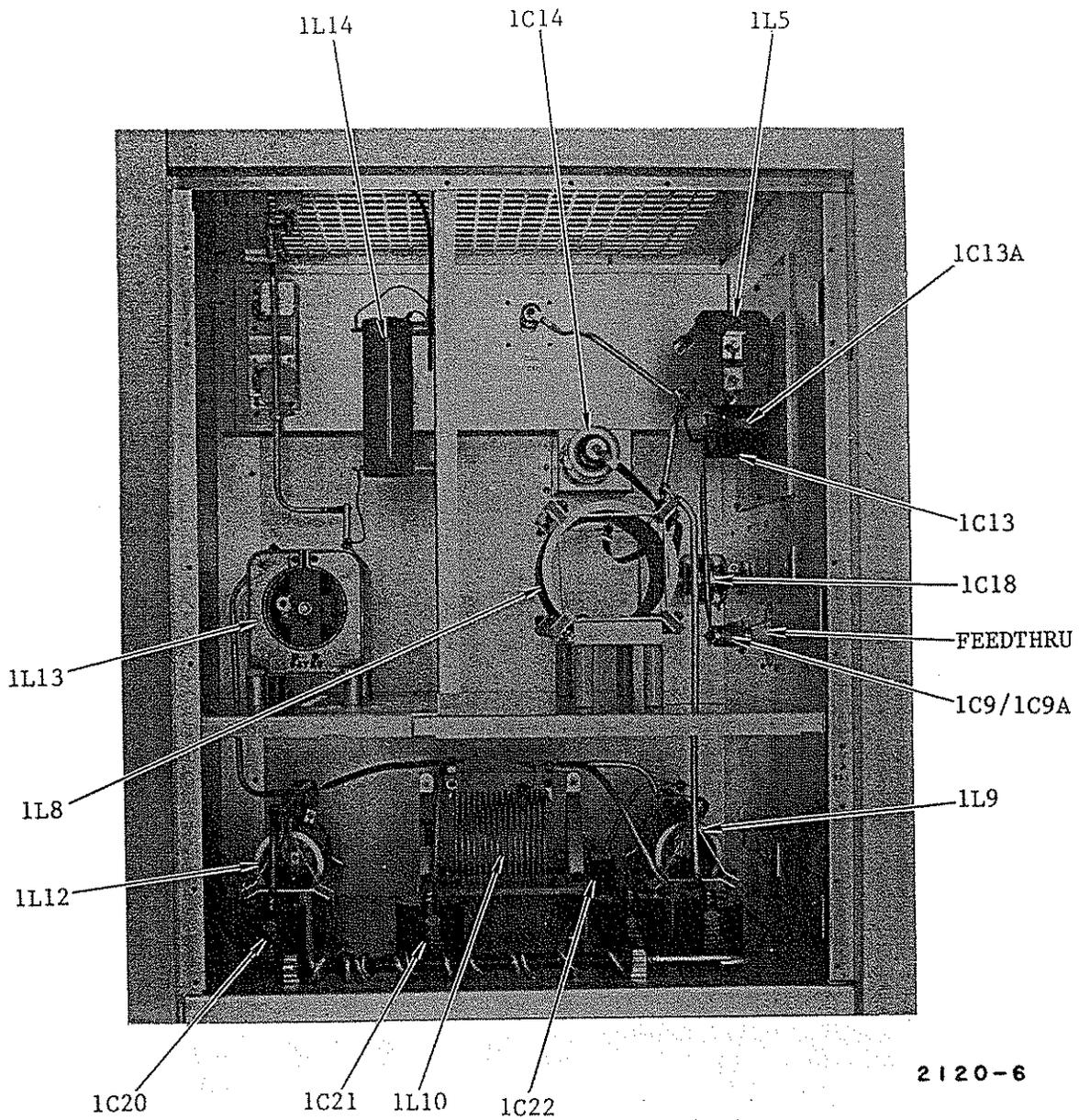
Figure 2-2. Transmitter Component Locations (Sheet 3 of 4)
