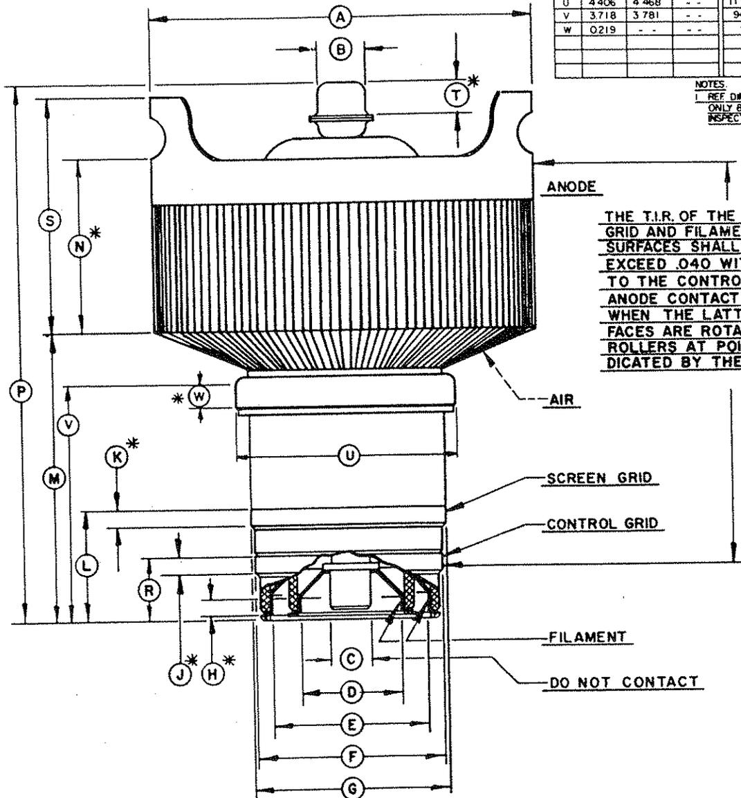
THE T.I.R. OF THE SCREEN GRID AND FILAMENT CONTACT SURFACES SHALL NOT EXCEED .040 WITH RESPECT TO THE CONTROL GRID AND ANODE CONTACT SURFACE WHEN THE LATTER SURFACES ARE ROTATED ON ROLLERS AT POINTS INDICATED BY THE ARROWS
